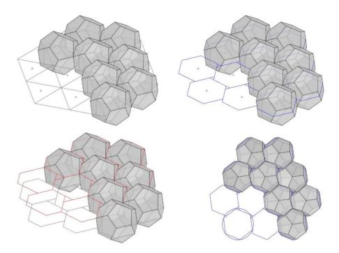
Fig. 2: Topological interlocking of pentagonal dodecahedra.
